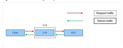
Figure 4-2 Load balancing at Layer 7
